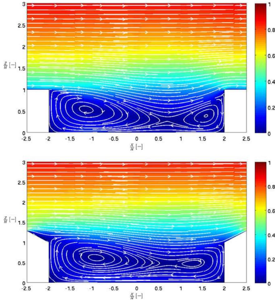
**Fig. 5.** Mean velocity magnitude,  $U$ , made non-dimensional by the free-stream velocity,  $U_f$ , (color map) for  $H/W=0.25$ . Flat roof case on the left and  $30^\circ$  roof slope on the right. Streamlines are drawn in white.
