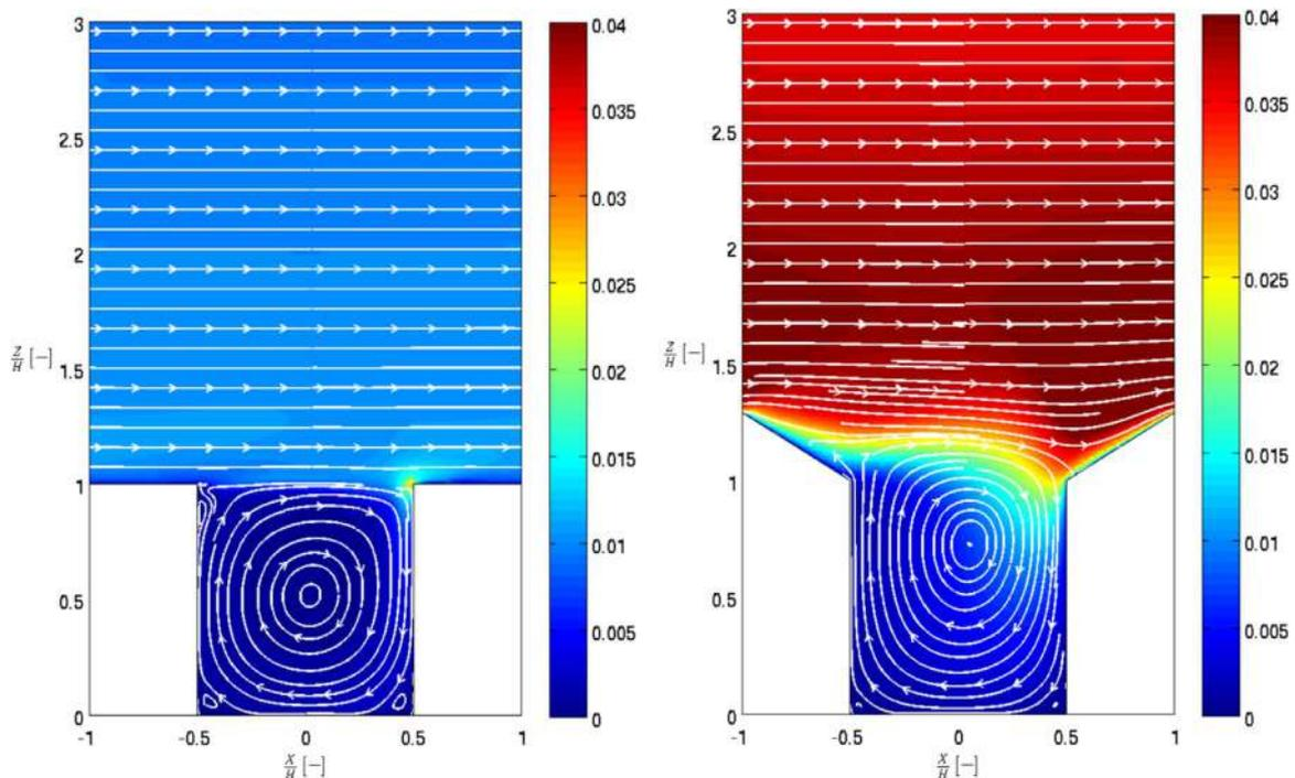
**Fig. 7.** Turbulent kinetic energy,  $k$ , made non-dimensional by the squared free-stream velocity,  $U_f^2$ , (color map) for  $H/W=1.00$ . Flat roof case on the left and  $30^\circ$  roof slope on the right. Streamlines are drawn in white.
