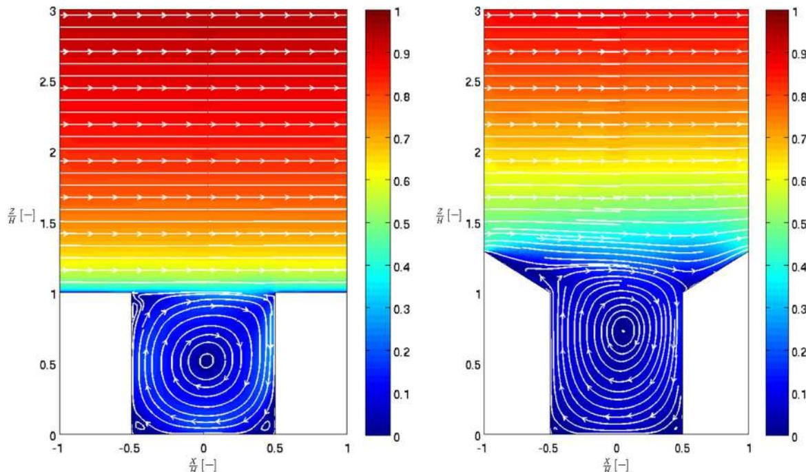
**Fig. 4.** Mean velocity magnitude,  $U$ , made non-dimensional by the free-stream velocity,  $U_f$ , (color map) for  $H/W=1.00$ . Flat roof case on the left and  $30^\circ$  roof slope on the right. Streamlines are drawn in white.
