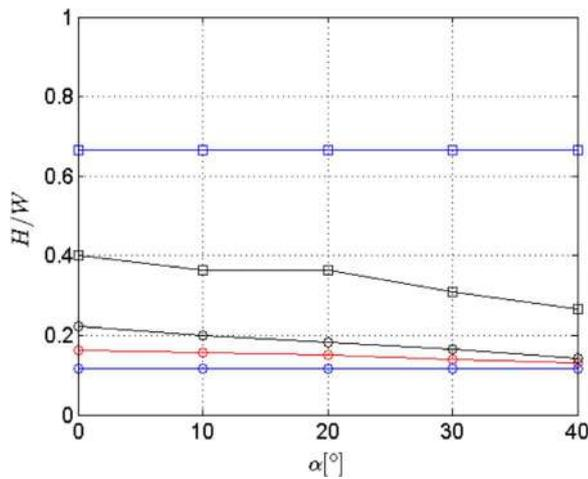
Fig. 14. Aspect ratios,  $H/W$ , of regime transition for different roof slopes. Squares indicate transitions from Skimming-Flow to Wake-Interference regime; circles indicate the transition from Wake-Interference to Isolated-Roughness. Transitions identified by the structure of the velocity field are plotted in black; transitions identified by  $C_{pW}$  slope are plotted in blue. Red line indicates the aspect ratios corresponding to the maximum friction coefficient.
