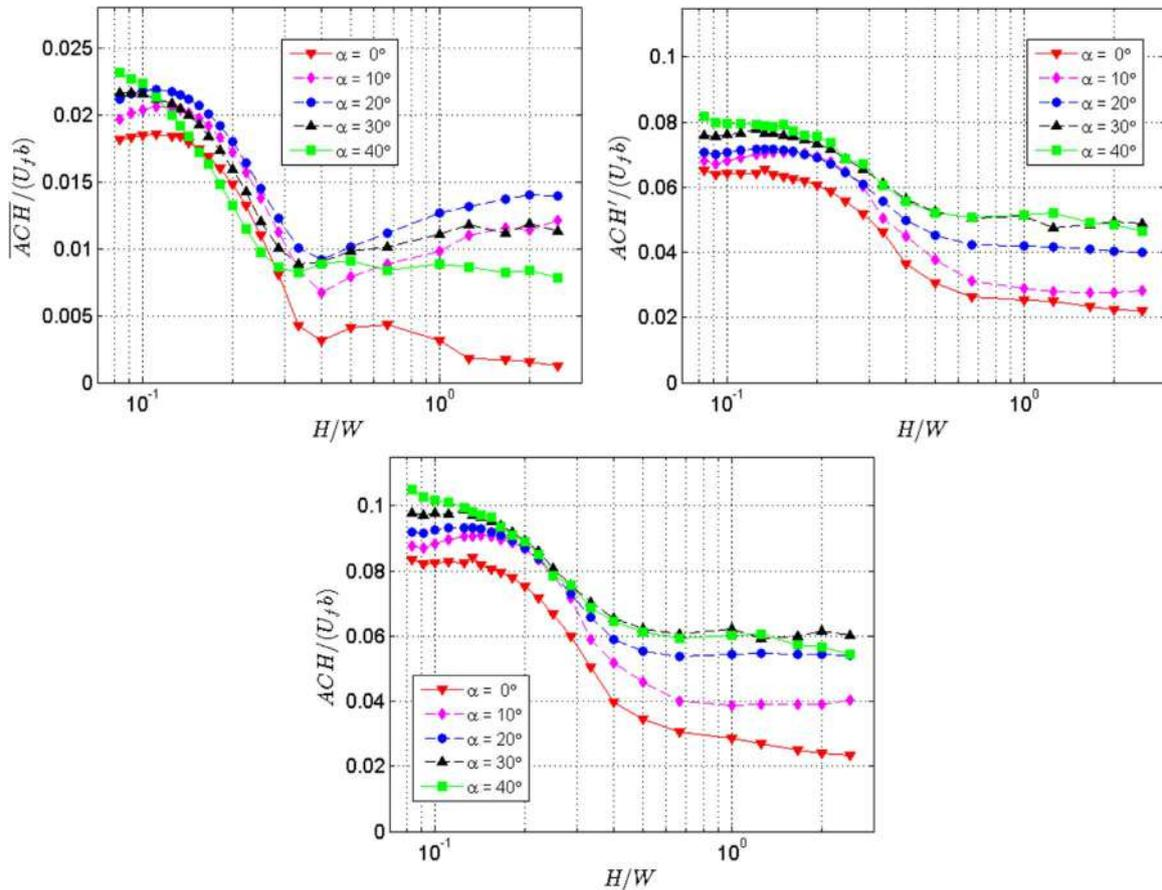
Fig. 10. Non-dimensional ACH components versus the UC aspect ratio,  $H/W$ , for different roof slopes (mean component: top left panel; turbulent component: top right panel; total ACH: bottom panel).
