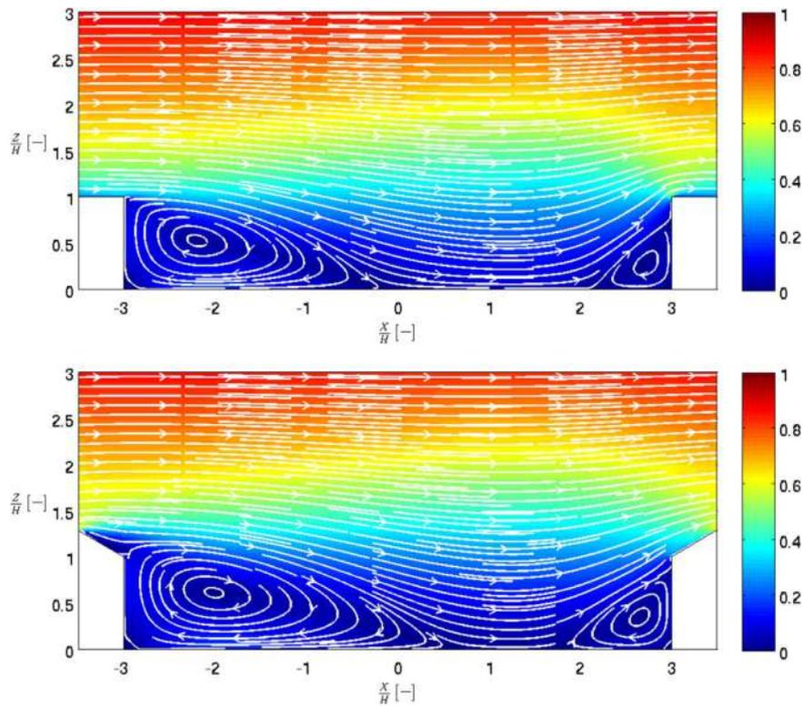
**Fig. 6.** Mean velocity magnitude,  $U$ , made non-dimensional by the free-stream velocity,  $U_f$ , (color map) for  $H/W=0.17$ . Flat roof case on the left and  $30^\circ$  roof slope on the right. Streamlines are drawn in white.
