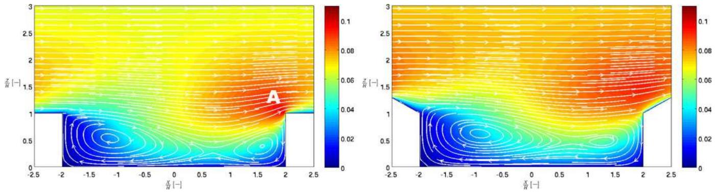
Fig. 8. Turbulent kinetic,  $k$ , energy made non-dimensional by the squared free-stream velocity,  $U_f^2$ , (color map) for  $H/W=0.25$ . Flat roof case on the left and  $30^\circ$  roof slope on the right. Streamlines are drawn in white.
