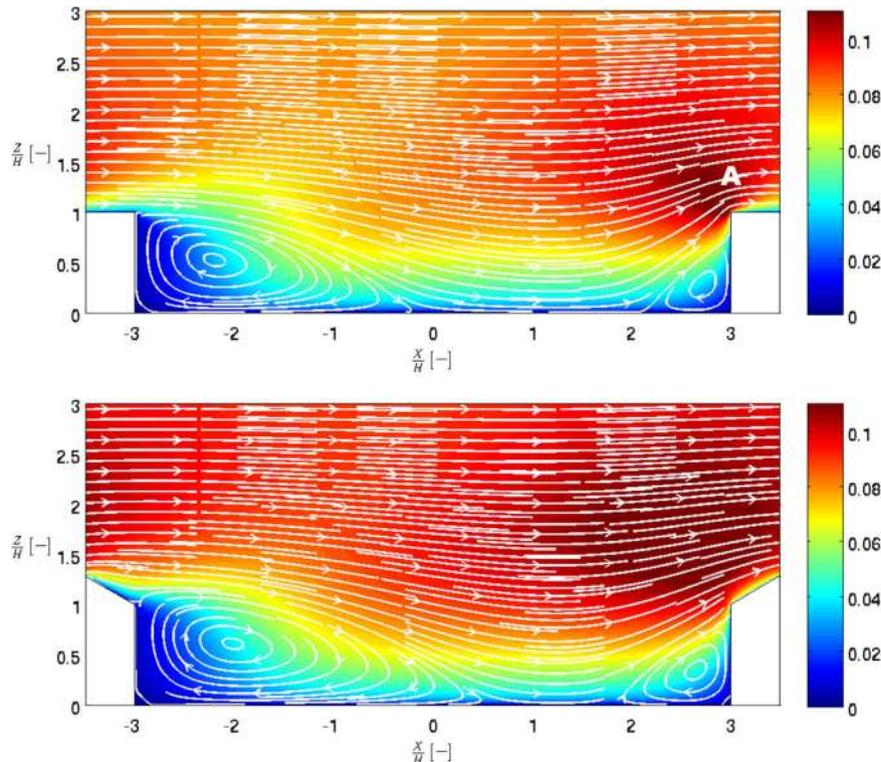
Fig. 9. Turbulent kinetic energy,  $k$ , made non-dimensional by the squared free-stream velocity,  $U_f^2$ , (color map) for  $H/W=0.17$ . Flat roof case on the left and  $30^\circ$  roof slope on the right. Streamlines are drawn in white.
