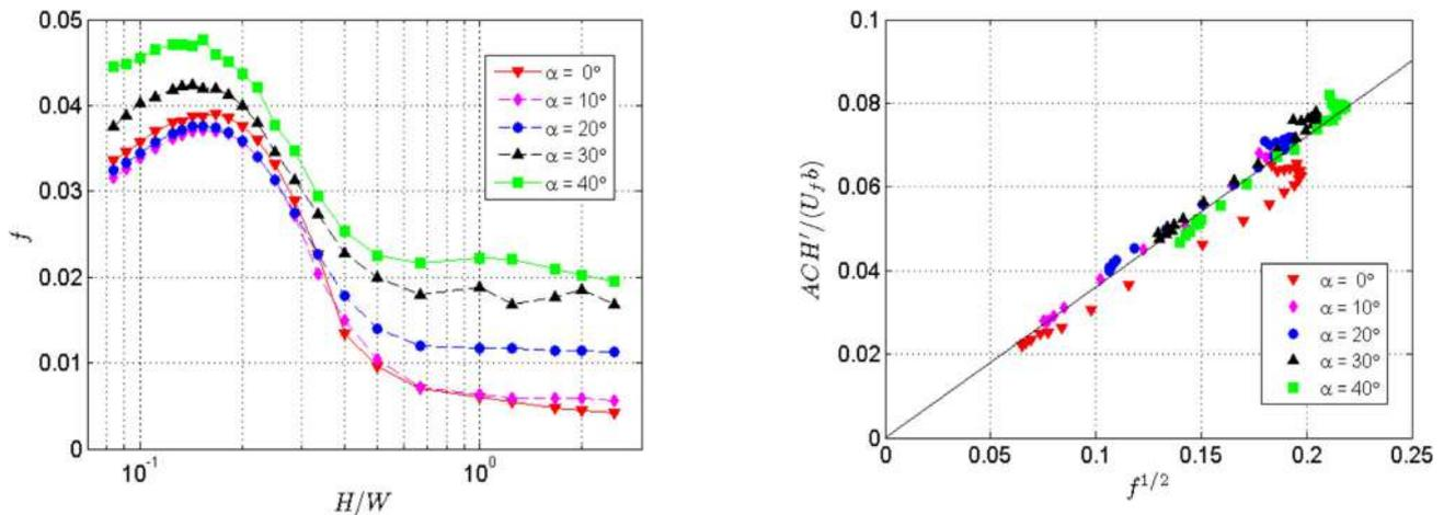
Fig. 11. Friction coefficient,  $f$ , as a function of the UC aspect ratio,  $H/W$ , for different roof slopes.
