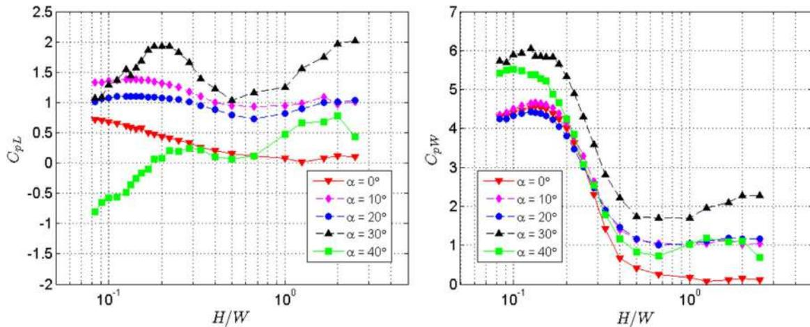
Fig. 13. Left panel: pressure coefficients at the leeward wall,  $C_{pL}$  (left panel), and windward wall,  $C_{pW}$  (right panel), versus  $H/W$  for different roof slopes.
