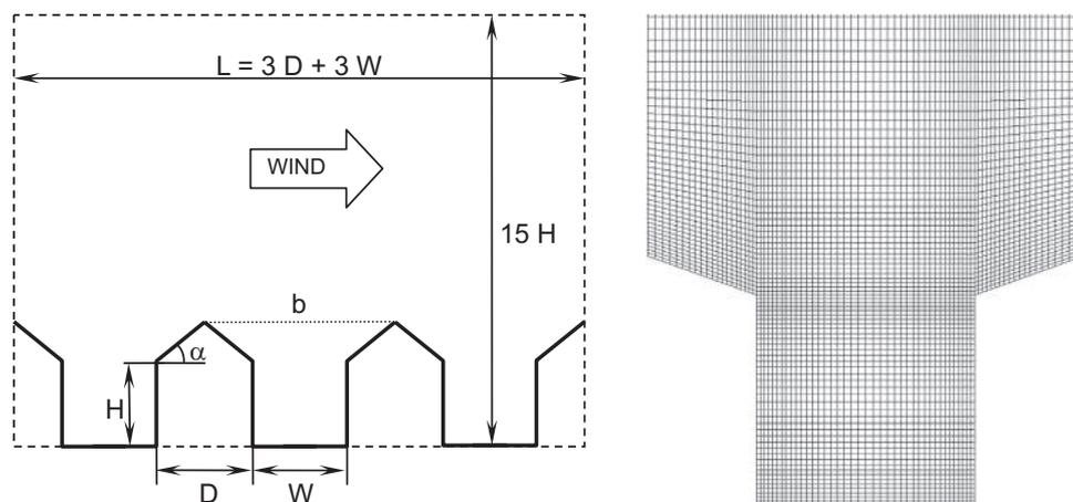
Fig. 1. Sketch of the computational domain:  $H$  is the eave height,  $D$  the width of the building,  $\alpha$  the roof slope,  $W$  the canyon width,  $L=3(D+W)$  the streamwise dimension of the domain, and  $b$  the line connecting the ridges (left panel). Inset of the mesh used for  $H/W=1$  and  $\alpha=20^\circ$  (right panel).
